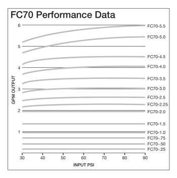
Note: This data is a schematic representation of the nominal flow performance for the FC70 under normal operating conditions. All elastomeres are subject to slight changes in flow due to water temperature, line pressure and/or differential pressure. More exacting flow information may be obtained by calling for technical assistance.
